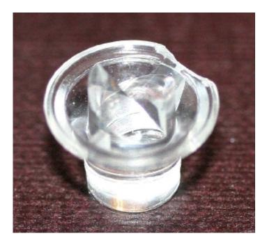
Prism used to measure eye pressure (Goldmann tonometry).
